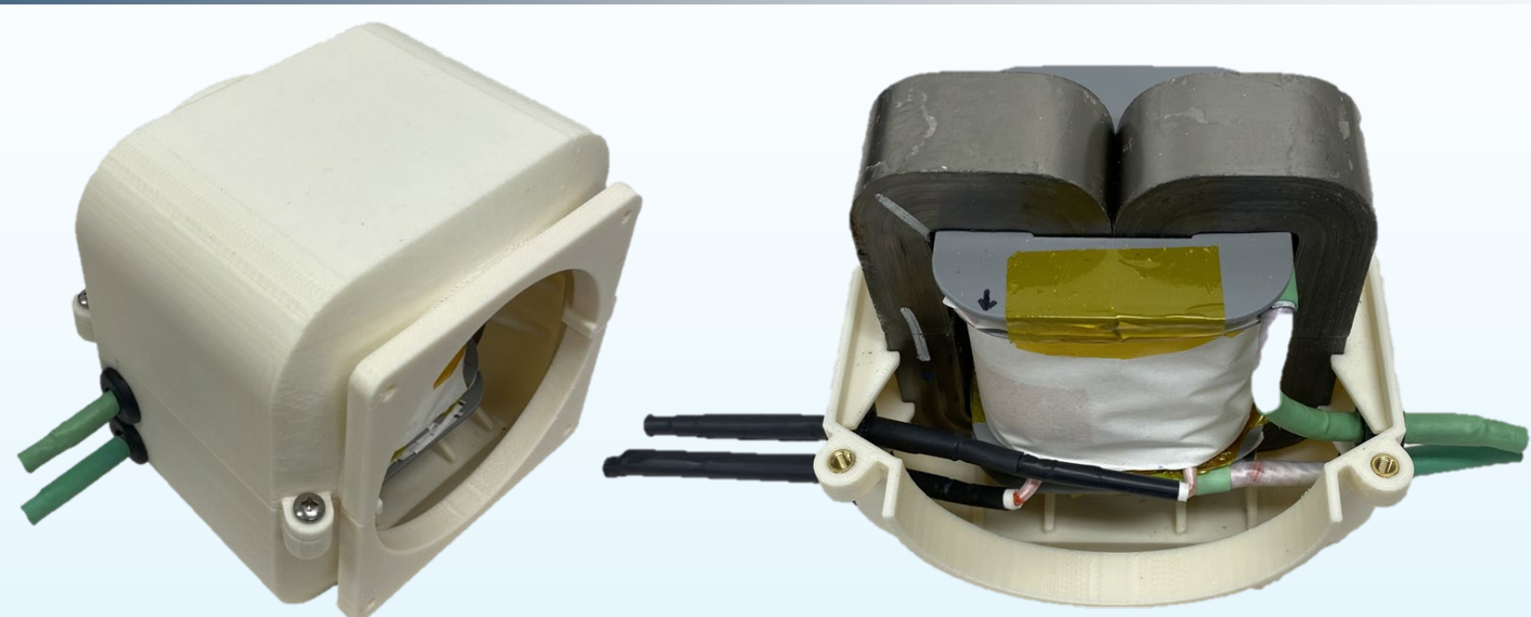
Figure 6. Baseline prototype with maximization window area utilization for reduced material utilization and cost.
