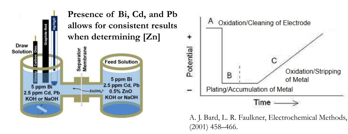
Anodic stripping voltammetry (ASV) allows for much faster screening of separators compared to ICP-MS, with similar limits of detection. ASV Analysis of Zn performed for the first time in alkaline conditions. J. Duay, T.N. Lambert, R. Aidun, *Electroanalysis*, 29 (2017) 1-8.
