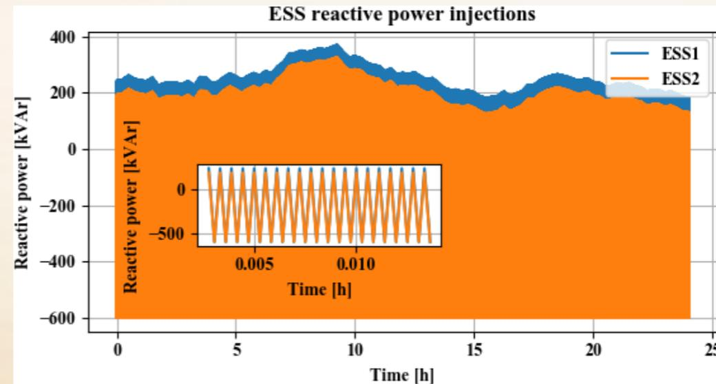
Resulting oscillations (stability loss) from volt-var control based on IEEE 1547-2018
