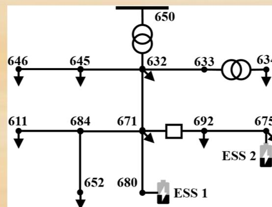
Sample 13-bus system to study effect of multiple droop controllers
